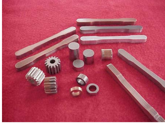
Fig. 5 Net-Shape Quality of CDC Processed Samples(e.g., Dogbones, Cylinders, Rings, & Gears)
