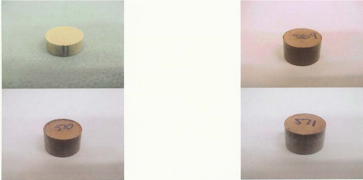
Fig. 9. Net Shape Fabrication Potential for Aluminum Nitride and Cu/AlN Ceramic Composite Cylinders (0.5 inch Diameter) [27]
