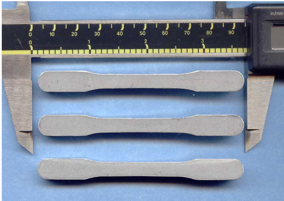
Fig. 10 As Compacted CDC-Green Al-3Mg Samples; Lubricant: Zinc Stearate Samples:A: #362 (30tsi);B: #364 (50tsi);C: #371 (150tsi)
